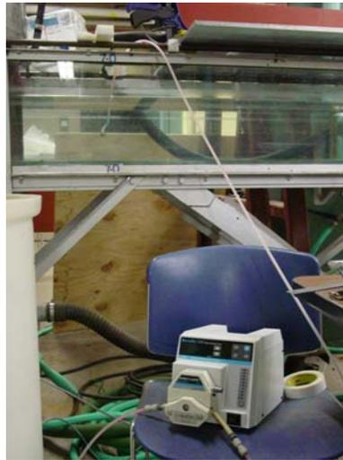
Figure 2.19: Dye injection for LIF.
