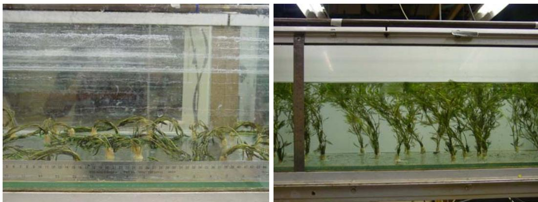
Figure 2.8: Stems attached to the bottom. (1) while being attached, (2) once the tank was filled up.
