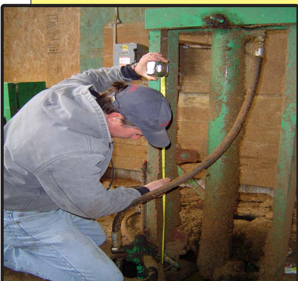
Measuring stroke length during Pump Calibration test
