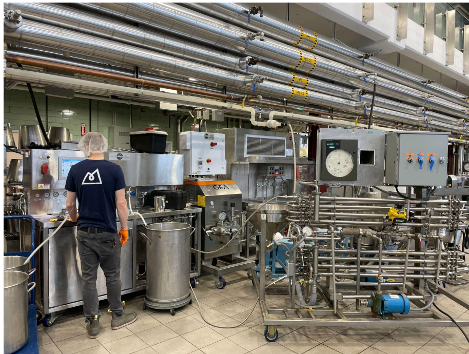
Figure 2.2: Microthermics and holding tube set-up
