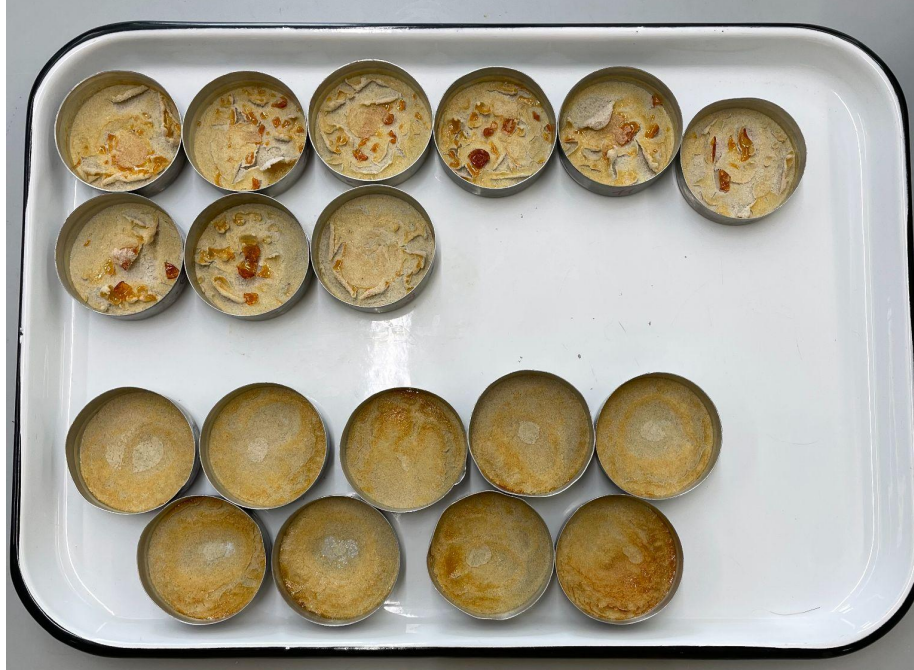
Figure 3.13: Samples after drying at 100°C for at least 12 hours. Top is pellet and the bottom is supernatant.
