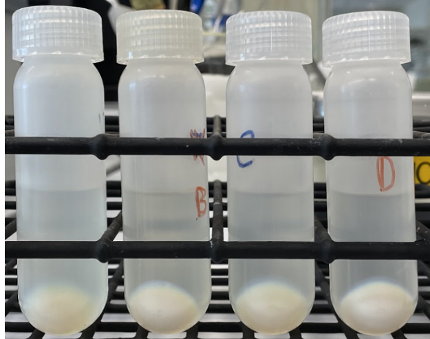
Figure 3.10: WPI/Casein solutions after successful centrifugation
