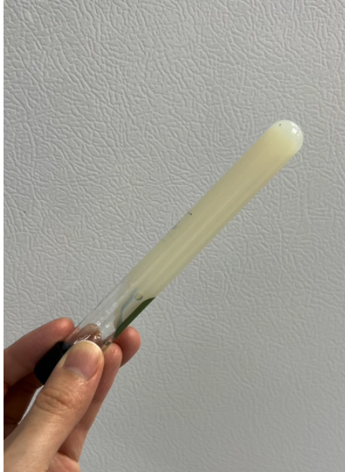
Figure 3.8: Failure of heated WPI/Casein solutions of 11%, pH 6.4
