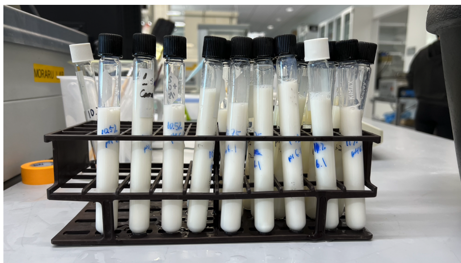
Figure 3.3: (from the left) Heated WPI/Casein solutions of 10.5% pH 6.1, 10.5% pH 6.2, 10.5% pH 6.3, 10.5% pH 6.4, 10.75% pH 6.1, 10.75% pH 6.2, 11% pH 6.1
