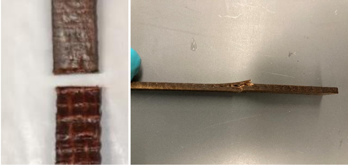
Figure 25: Tensile fracture of a JF/(0/100) wGA hybrid composite (left) and tensile fracture of a GA-free JF/(30/70) hybrid composite (right)
