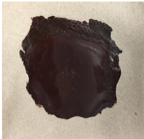
Figure 18: A 0/100 wGA resin post hot pressing
