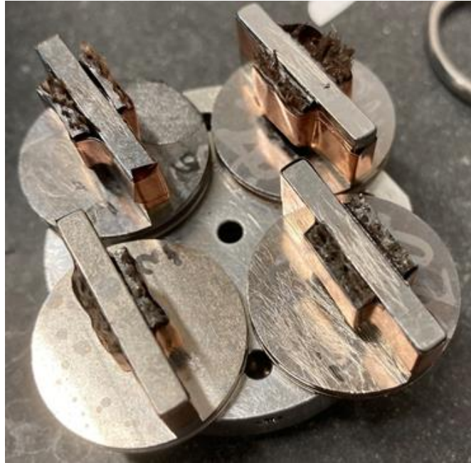
Figure 7: Au/Pd coated JF/(CFF/SPI) composite specimens loaded for SEM analysis
