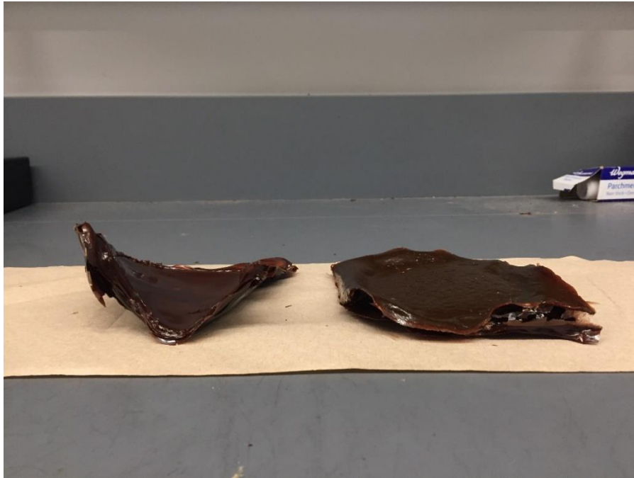
Figure 21: CFF/SPI resin specimens prior to hot pressing: (left) 0/100 wGA and (right) 10/90 wGA
