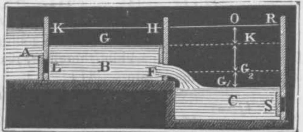
Let the mean horizontal transverse section of a simple lock chamber =  $G$ , the distance of the middle of the sluice in the upper gate from the upper surface  $HR$  of the upper reach =  $h_1$ , and from that of the lower reach =  $h_2$ , and, lastly, the area of the aperture or sluice opening =  $F$ , we then obtain the time of filling up to the middle of the
