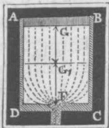
It is seen from the formula  $v_1 = \sqrt{2 \left( \frac{\mu F}{G} \right)^2 g x}$ , that the motion of the surface is uniformly retarded, and the measure of the retardation  $p = \left( \frac{\mu F}{G} \right)^2 g$ , hence we also know (§ 14), that this velocity = 0, and the discharge ceases, when
