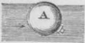
and have an opening with a neck, that they may be filled with water and stopped. A floating ball, such as  $A$ , Fig. 510, gives only the velocity at the surface, and often only that of the main current; but by sus-
