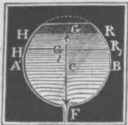
$$\begin{aligned} t &= \frac{1}{3} \cdot \frac{\pi r h^3}{\mu F \sqrt{2gh}} = \frac{2}{3} \cdot \frac{\pi h^3}{\mu F \sqrt{2gh}} \\ &= \frac{2}{15} \pi \frac{(10r - 3h) h^3}{\mu F \sqrt{2g}}, \end{aligned}$$
