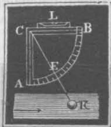
For velocities under four feet we may use the ivory ball, but for greater velocities the hollow metal ball. On account of the constant undulations of the ball in the direction of the motion of the water, as also at right angles to the direction of the current, the reading off is somewhat difficult, and leaves a good deal of uncertainty, for which reason this instrument cannot be relied upon for the more exact numbers.
