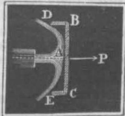
§ 387. *Impulse of a Limited Stream.*—If we add borders *BD*, *CE*, to the perimeter of a plane surface *BE*, Fig. 527, which project from the side impinged upon by the water, then will the water deviate from its direction at an obtuse angle, in a similar manner as from
