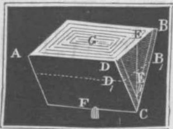
time of efflux may be found in the following manner. Let us divide the height  $CE = h$  into  $n$  equal parts, and carry horizontal planes through the points of division; let us then decompose the whole quantity of water into equally thick strata of equal length  $AD = l$ , and of breadths diminishing downwards. If the breadth of the upper stratum  $BD = b$ , we have then the breadth of another stratum  $D_1B_1$ ,
