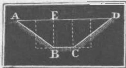
In every case the angle of slope  $B\hat{A}E = \theta$ , Fig. 498, or the slope  $n = \frac{AE}{BE} = \cotang. \theta$  may be regarded as a given
