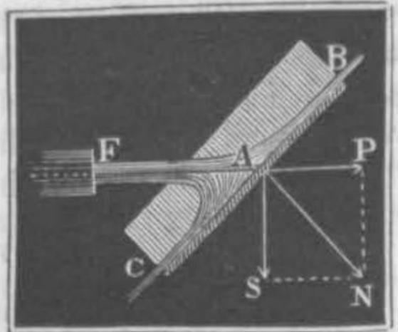
But if the impinged plane  $BC$ , Fig. 530, is only bordered on two oppositely situated sides, the stream then divides itself into two unequal portions; the greater portion  $Q_1$  takes the small deflexion  $\alpha$ , and the lesser  $Q_2$ , the greater deflexion  $180 - \alpha$ ; hence, the whole impulse in the direction of the stream is
