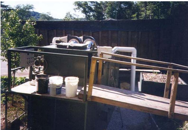
*In-vessel composting unit with biofilter.*
