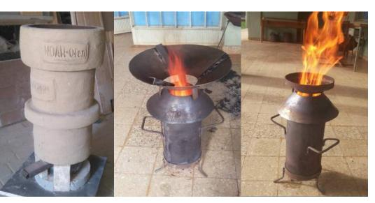
Figure 7: Pro Lehm Clay gasifiers stoves (left) and Elsa metal gasifier stoves with different pot raiser (Venkata et al. 2016)
