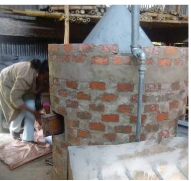
**Figure 15.** Furnace for biochar production from bamboo (Copyright: Tarikayehu Gebresilassie)
