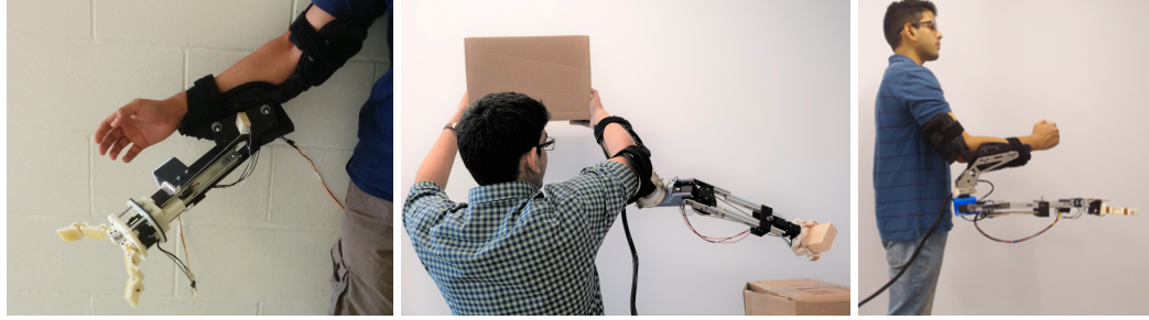
Figure 1.2: Successive wearable robotic forearm prototypes: Models I, II, and III (left to right).
