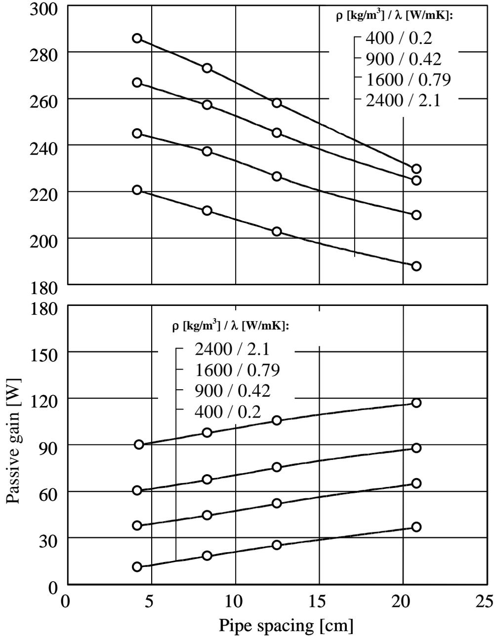
Figure 3. Amount of active gain (upper diagram) and passive gain (lower diagram), dependent on thermal properties of the wall and pipe spacing.
