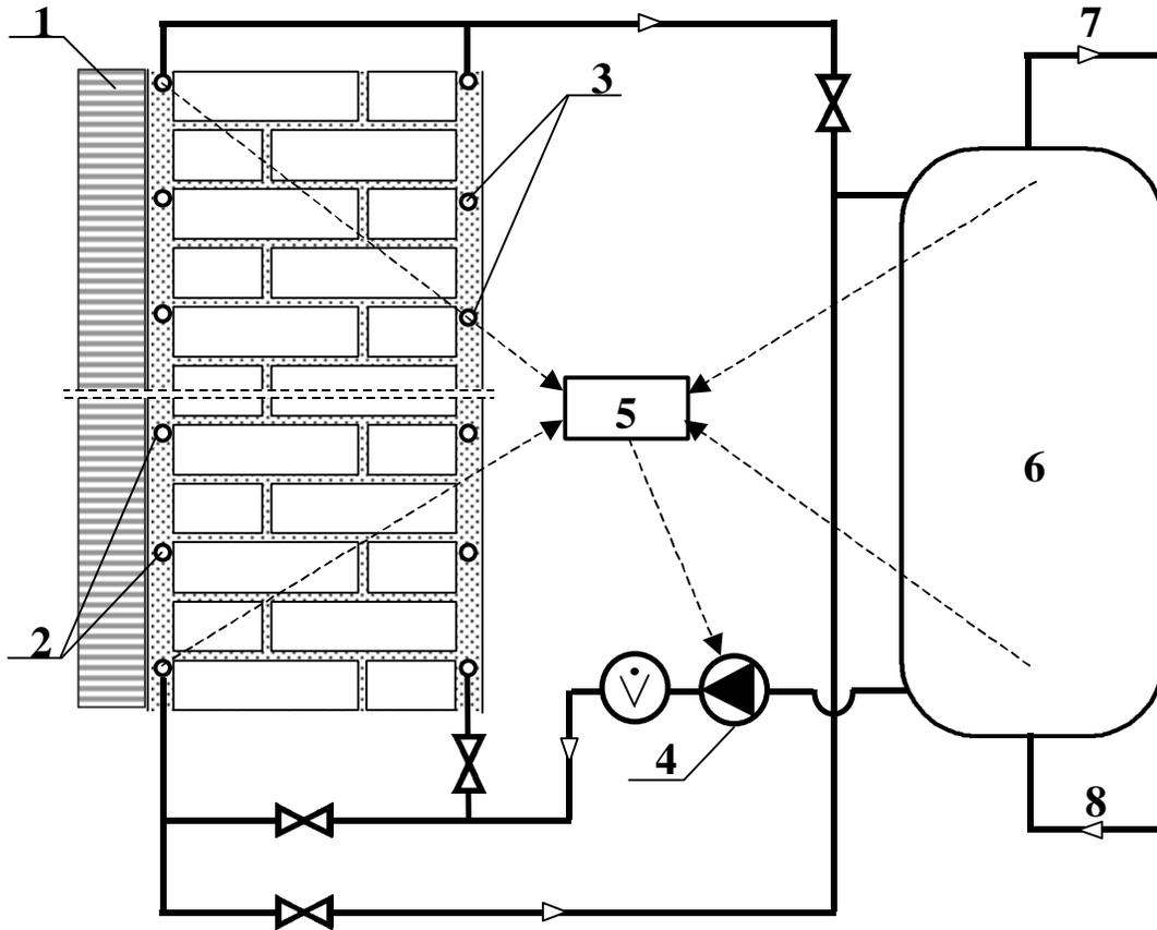
Figure 1. Hybrid wall scheme: 1- transparent thermal insulation, 2 – outer piping, 3- inner piping, 4- water pump, 5 – pump controller, 6 – water tank, 7 – hot water outlet, 8 – cool water inlet.
