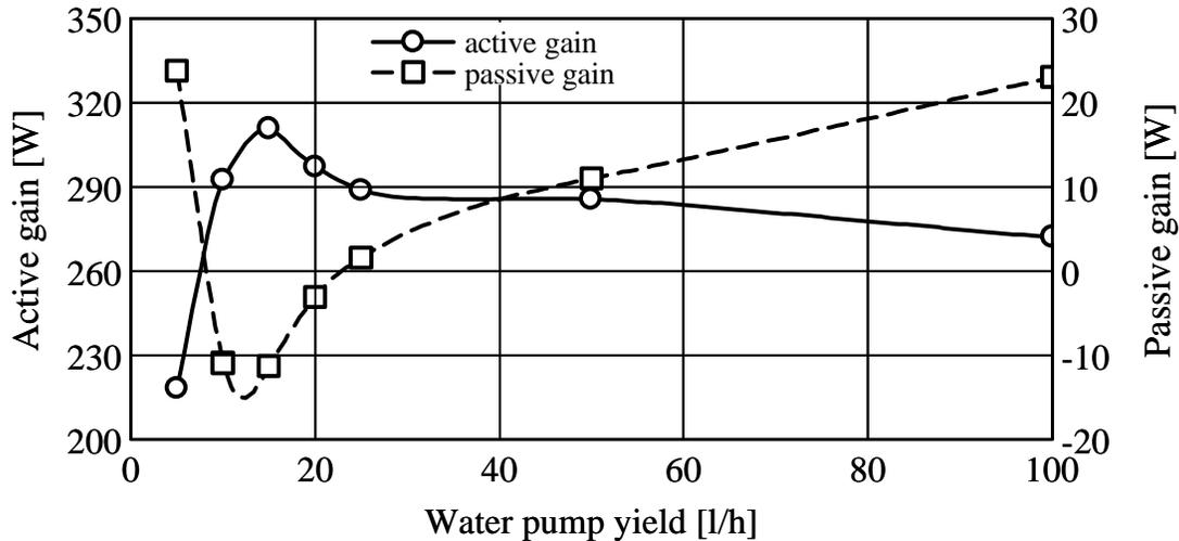
Figure 5. Relation between water pump yield and amounts of active and passive gain.
