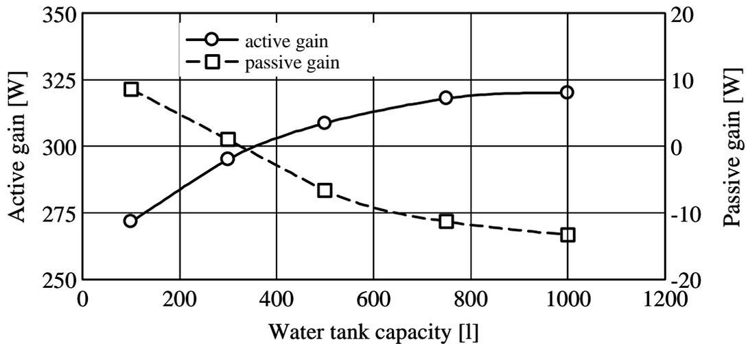
Figure 4. Relation of passive and active gain to water tank capacity.
