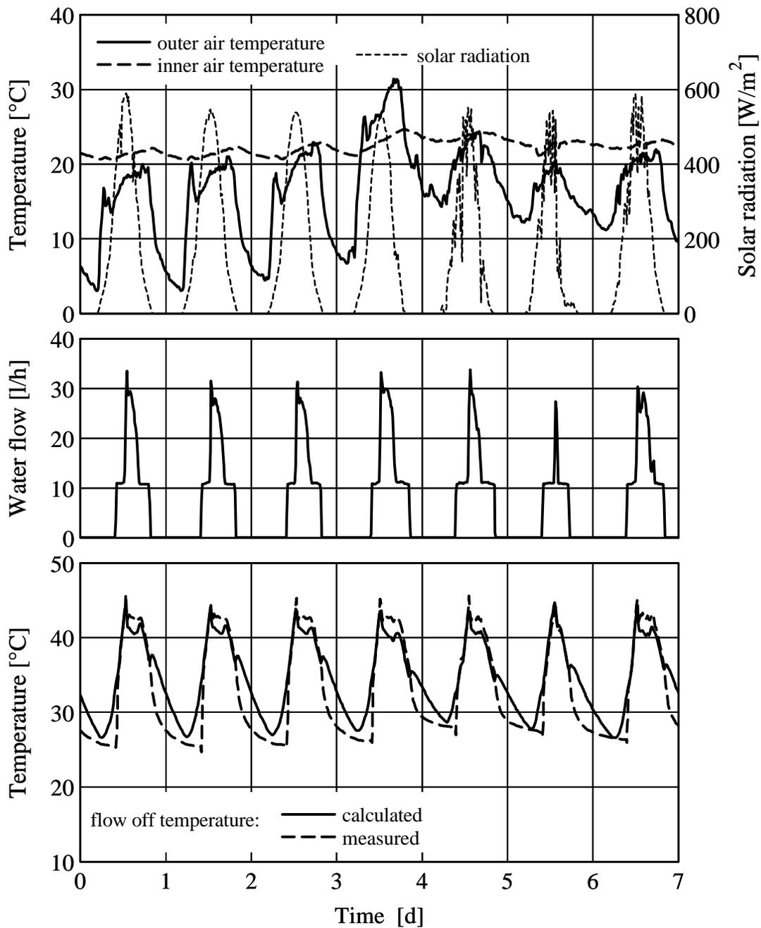
Figure 2. Boundary conditions (upper diagram), measured water flow (middle diagram) and measured and calculated water temperature at the outlet, in the period between 20 July – 26 July 1997.
