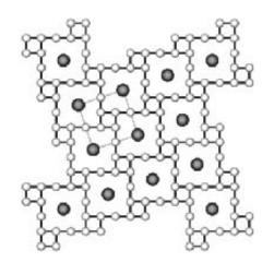
The pattern of the CsTe<sub>6</sub> sheet (fig. 2), looking down the c-axis onto the sheet; the darker and larger spheres are Cs, the light ones (Te) is remarkable. This is a net of rare symmetry containing only fourfold and twofold rotation axes.
