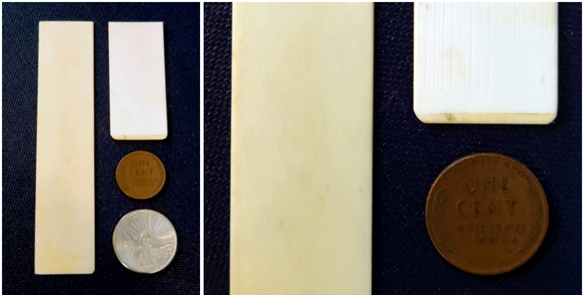
Figure 25a, b: Two ivory veneers from keyboard pictured above. Left key: obverse high C (single long strip of ivory); right key: smaller end, reverse, showing scoring to attach glue and fabric and incision at bottom to fit ivory facing. For scale: 2022 Maya Angelou quarter (reverse), 1947 wheat penny (reverse). Photos: author, April 2022.
