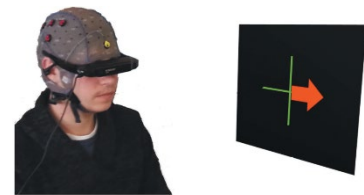
[fig18] User setup with a HMD and an EEG cap with the electrodes over the motor and sensorimotor cortices, Vourvopoulos et al. (2016)
