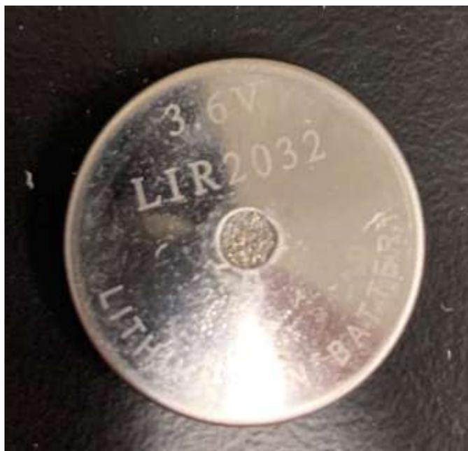
Figure 5-3. Picture of the DEMS coin cell cathode case
