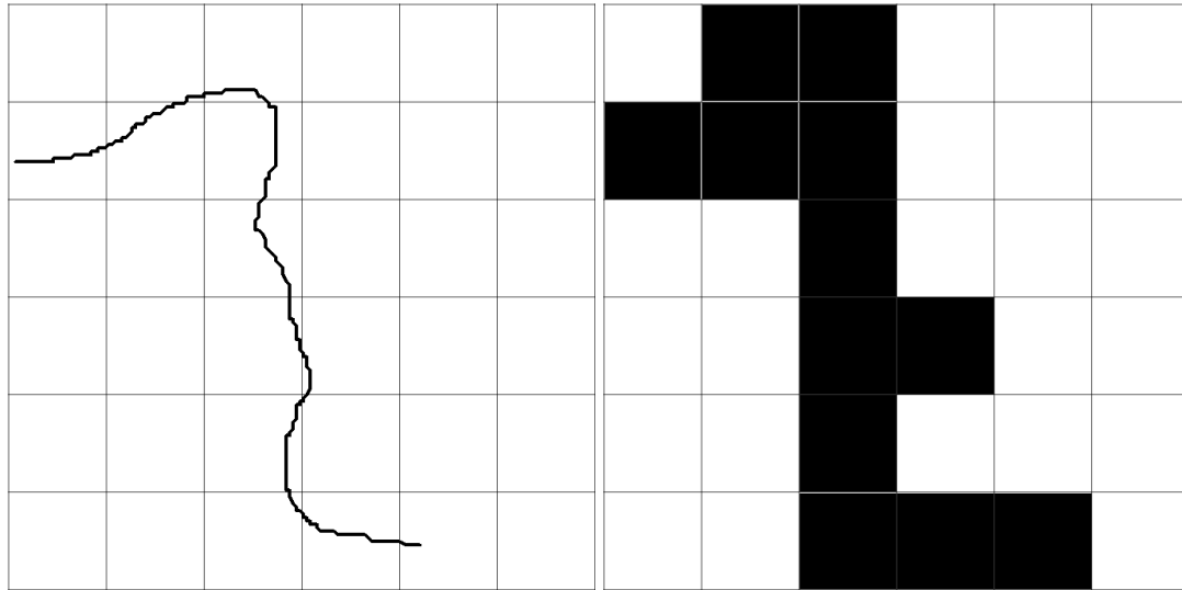
(a) The intended complicated stroke input (b) A potential raw input detected by the sensor onto a sensing grid.
