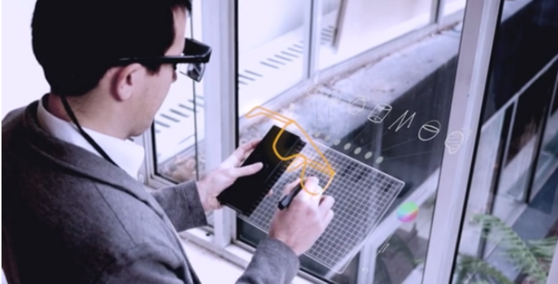
Figure 2.7: Augmented reality sketching using the Gravity tablet and headset. The tablet is used to define the location of the sketch plane in the “virtual” workspace, which can then be drawn upon. [22]
