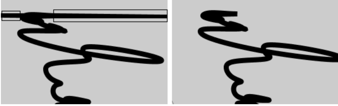
Figure 6.6: Left: An example of a miter join artifact from a sharp curve. The boxed regions show the artifact. Right: The artifact is detected by calculating the length of the miter join. If detected, the join is replaced with a bevel join.
