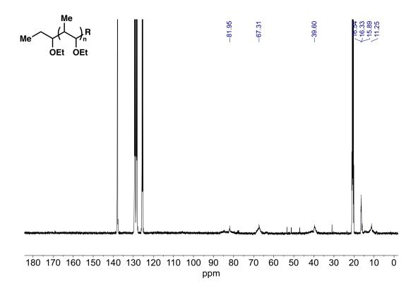
Figure 6.17.  $^{13}$ C NMR of poly(EPE) in d8-toluene at 80  $^{\circ}$ C (Table 6.1, entry 10).
