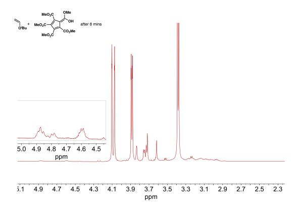
Figure 6.32. Zoom of <sup>1</sup>H NMR spectrum of the IBVE and PCCP mixture after eight minutes of reaction time; Insert highlights the appearance of new resonances between 4.5 and 5.0 ppm.
