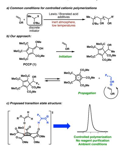
Figure 6.1. (a) Typical reaction conditions of cationic polymerizations. (b) PCCP is used in this work to controllably polymerize vinyl ethers. (c) Key H-bonding interactions lead to a controlled polymerization with narrow molecular weight distributions.
