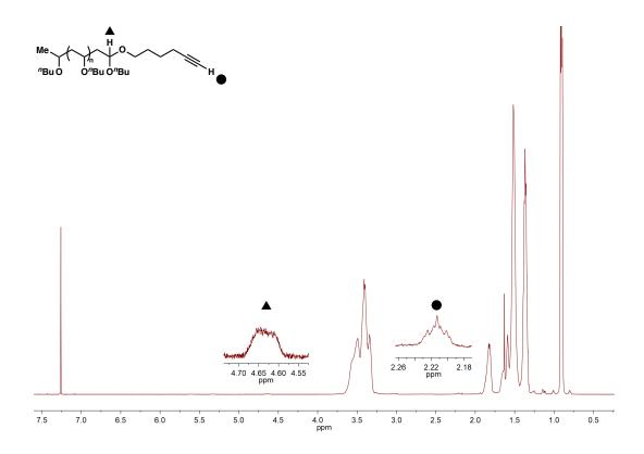
Figure 5.9. <sup>1</sup>H NMR of poly(*n*-butyl vinyl ether) functionalized with 5-hexyn-1-ol.
