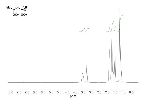
Figure 6.14. <sup>1</sup>H NMR of poly(CyVE) in CDCl<sub>3</sub> (Table 6.1, entry 9).
