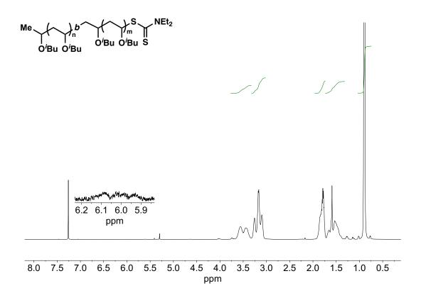
Figure 6.28. <sup>1</sup>H NMR of poly(IBVE-*b*-IBVE) functionalized with dithiocarbamate after chain extension using ferrocenium (Figure 6.4b).
