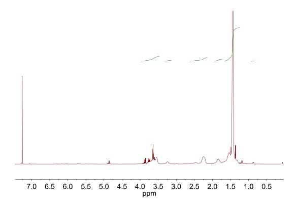
Figure 3.17. <sup>1</sup>H NMR of poly(2-chloroethyl vinyl ether-r-tert-butyl acrylate) ( $M_n$  = 13.8 kg/mol, D = 1.42,  $M_{n,theo}$  = 12.1 kg/mol).
