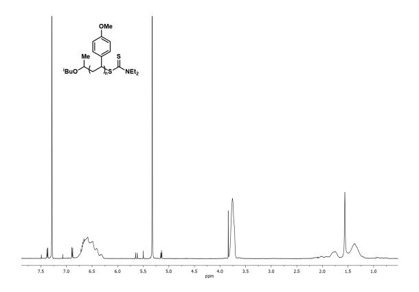
Figure 4.12. <sup>1</sup>H NMR of poly(p-methoxystyrene),  $M_n$  = 11.9 kg/mol,  $\theta$  = 1.21 (Table 4.2, entry 6).
