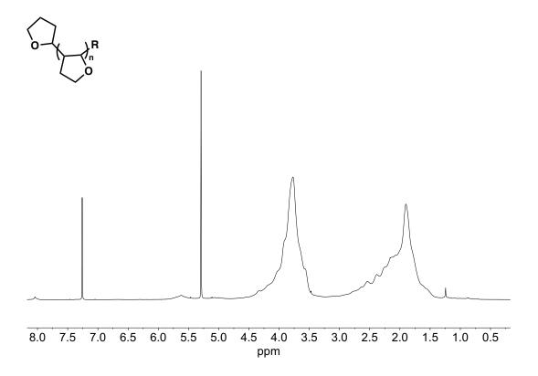
Figure 6.18.  $^{1}H$  NMR of poly(DHF) in CDCl<sub>3</sub> (Table 6.1, entry 12).
