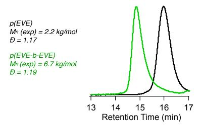
Figure 6.23. SEC traces of poly(EVE) and poly(EVE-b-EVE) synthesized under ambient conditions.
