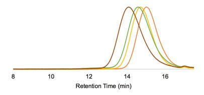
Figure 5.5. Representative GPC traces of poly(isobutyl vinyl ether) prepared by the general procedure above.
