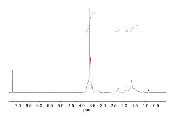
Figure 3.20. <sup>1</sup>H NMR of poly(2-chloroethyl vinyl ether-*co*-methyl acrylate) ( $M_n$  = 6.6 kg/mol,  $\mathcal{D}$  = 1.48,  $M_{n,theo}$  = 9.8 kg/mol).
