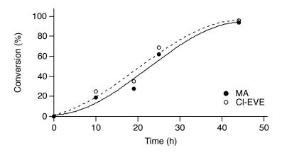
Figure 3.22. Multiblock copolymerization of methyl acrylate and 2-chloroethyl vinyl ether with  $Ir(ppy)_3$  and pyrylium.
