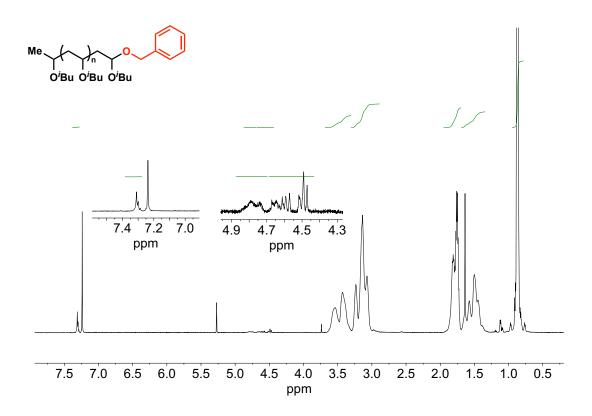
Figure 6.24. <sup>1</sup>H NMR of poly(IBVE) functionalized with 5-hexen-1-ol;  $M_n$  (GPC) = 5.4 kg/mol;  $M_n$  (NMR) = 6.6 kg/mol.
