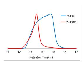
Figure 7.14. Size-exclusion chromatograms of polydisperse PS block and the corresponding PS-*b*-PI block copolymers corresponding to entry 7a in Figure 7.6.
