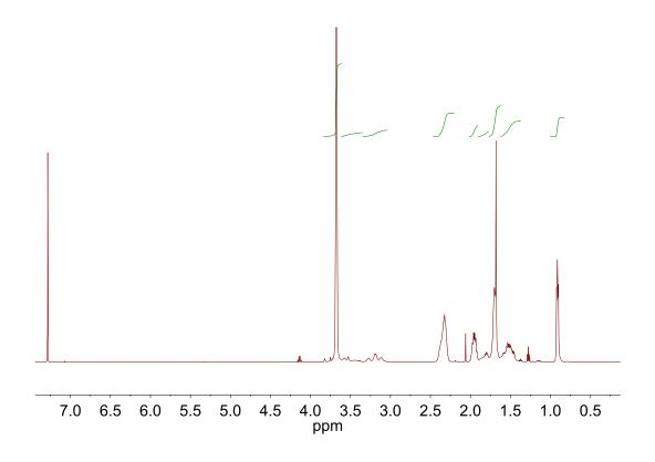
Figure 3.13. <sup>1</sup>H NMR of poly(isobutyl vinyl ether-*b*-methyl acrylate) (after purification)  $(M_n = 16.6 \text{ kg/mol}, D = 1.38, M_{n,\text{theo}} = 12.8 \text{ kg/mol}).$
