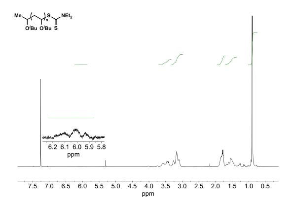
Figure 6.27. <sup>1</sup>H NMR of poly(IBVE) functionalized with dithiocarbamate prior to chain extension (Figure 6.4b).
