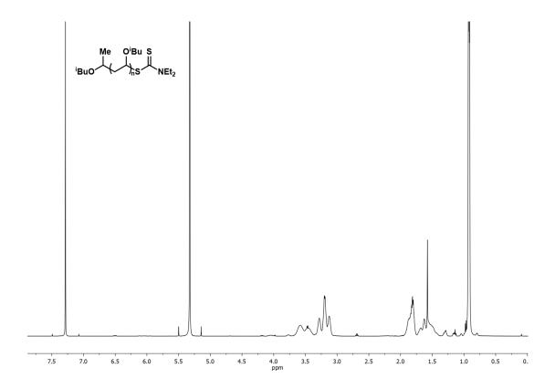
Figure 4.13. <sup>1</sup>H NMR of poly(isobutyl vinyl ether),  $M_n = 8.5$  kg/mol, D = 1.14.
