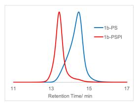
Figure 7.8. Size-exclusion chromatograms of polydisperse PS block and the corresponding PS-b-PI block copolymers corresponding to entries 1a,b in Figure 7.6.
