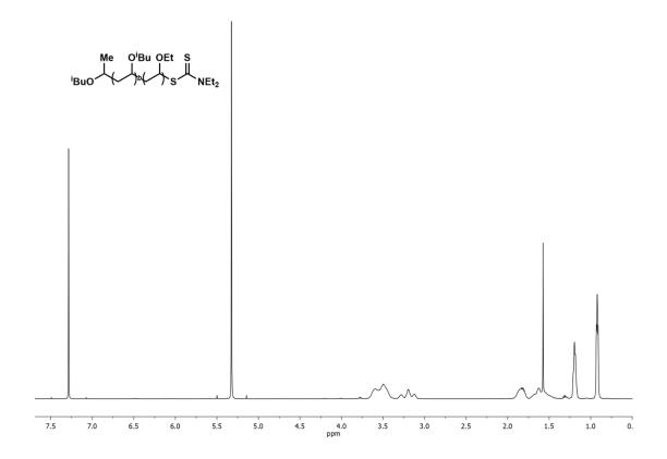
Figure 4.14. <sup>1</sup>H NMR of poly(isobutyl vinyl ether-*block*-ethyl vinyl ether),  $M_n = 13.4$  kg/mol, D = 1.09.
