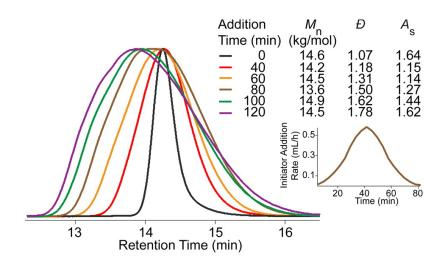
Figure 7.5. Size exclusion chromatography curves of a bell-shaped initiator addition profile. Inset: rate (mL/h) vs time (min) of an 80 min addition profile.
