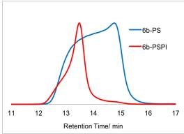
Figure 7.13. Size-exclusion chromatograms of polydisperse PS block and the corresponding PS-*b*-PI block copolymers corresponding to entries 6a,b in Figure 7.6.
