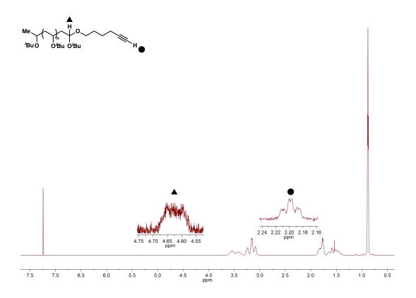
Figure 5.8. <sup>1</sup>H NMR of poly(isobutyl vinyl ether) functionalized with 5-hexyn-1-ol.
