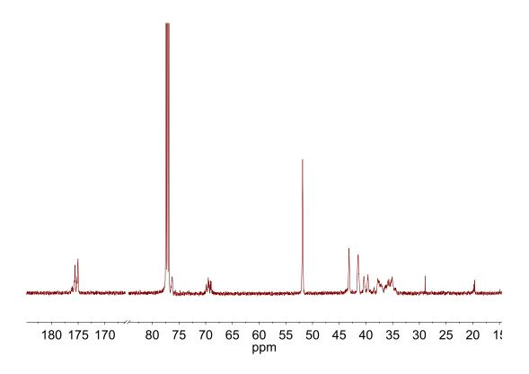
Figure 3.15.  $^{13}$ C NMR of poly(2-chloroethyl vinyl ether-r-methyl acrylate) ( $M_n$  = 6.5 kg/mol, Đ = 1.41,  $M_{n,theo}$  = 10.3 kg/mol).
