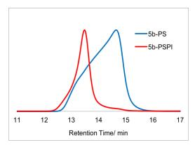
Figure 7.12. Size-exclusion chromatograms of polydisperse PS block and the corresponding PS-*b*-PI block copolymers corresponding to entries 5a,b in Figure 7.6.
