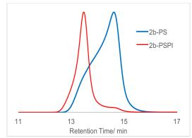
Figure 7.9. Size-exclusion chromatograms of polydisperse PS block and the corresponding PS-b-PI block copolymers corresponding to entries 2a,b in Figure 7.6.
