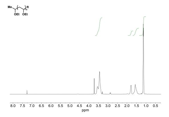
Figure 6.8. <sup>1</sup>H NMR of poly(EVE) in CDCl<sub>3</sub> (Table 6.1, entry 5).
