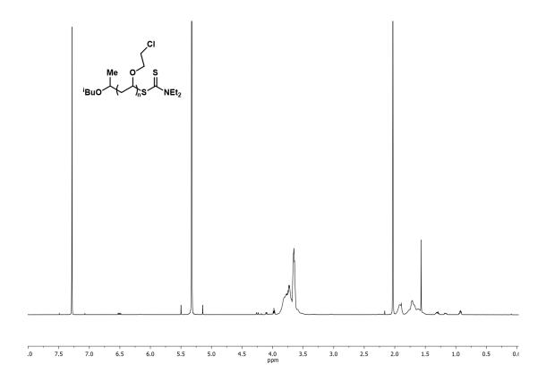
Figure 4.10.  $^{1}$ H NMR of poly(2-chloroethyl vinyl ether),  $M_{\rm n}$  = 7.8 kg/mol,  $\theta$  = 1.14 (Table 4.2, entry 4).
