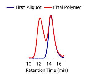
Figure 4.16. GPC Traces of Chain Extension from p(MA) Synthesized in the absence of IBVE.
