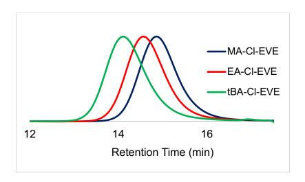
Figure 3.19. GPC traces of acrylate-2-chloroethyl vinyl ether copolymers (data from Table 3.1).
