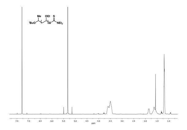
Figure 4.9. <sup>1</sup>H NMR of poly(ethyl vinyl ether),  $M_{\rm n}$  = 6.9 kg/mol,  $\theta$  = 1.06 (Table 4.2, entry 3).
