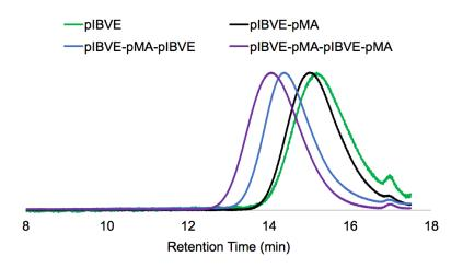
Figure 4.19. GPC traces of p(IBVE-b-MA-b-IBVE-b-MA) (Figure 6d)
