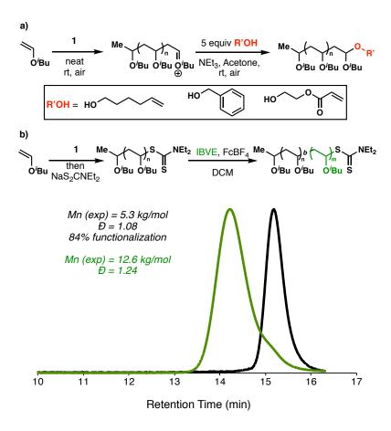
Figure 6.4. *In situ* chain-end functionalization of poly(IBVE) by quenching the polymerization (a) with functional alcohols and (b) with a dithiocarbamate salt, followed by chain extension with IBVE using ferrocenium tetrafluoroborate as the initiator.
