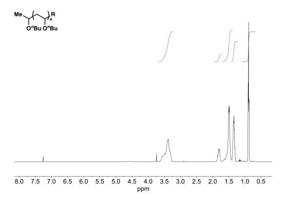
Figure 6.10. <sup>1</sup>H NMR of poly(NBVE) in CDCl<sub>3</sub> (Table 6.1, entry 7).
