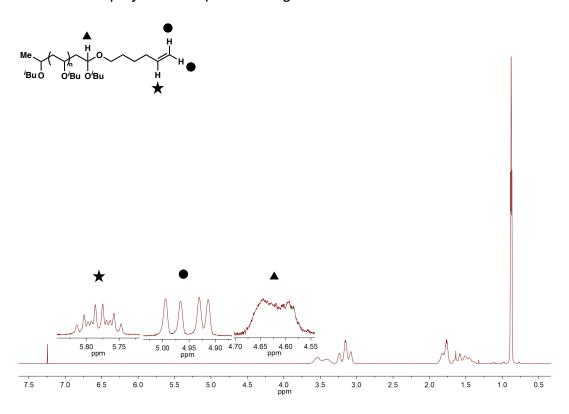
Figure 5.6. <sup>1</sup>H NMR of poly(isobutyl vinyl ether) functionalized with 5-hexen-1-ol.
