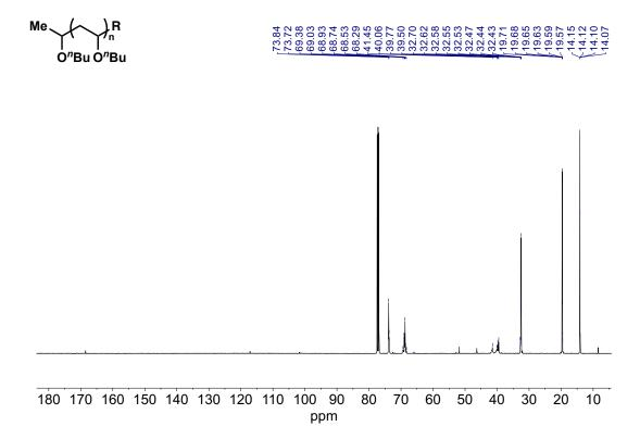
Figure 6.11. <sup>13</sup>C NMR of poly(NBVE) in CDCl<sub>3</sub> (Table 6.1, entry 7).
