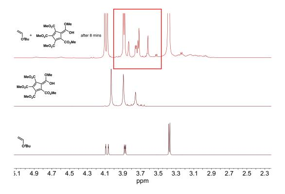
Figure 6.31. Zoom of stacked <sup>1</sup>H NMR spectra of IBVE, PCCP (1), IBVE and PCCP mixture after eight minutes of reaction time (bottom to top). Red box highlights new methyl-ester resonances of 1 upon reaction with IBVE.
