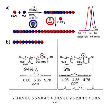
Figure 4.5. (a) A random copolymer of MA and IBVE can act as a macroinitiator for poly(MA-*b*-IBVE). (b) <sup>1</sup>H NMR chain-end analysis of the random copolymer revealed >90% thioacetal chain-ends.
