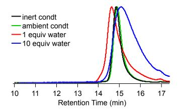
Figure 6.29. SEC traces of poly(IBVE) synthesized in the presence of different amounts of water.
