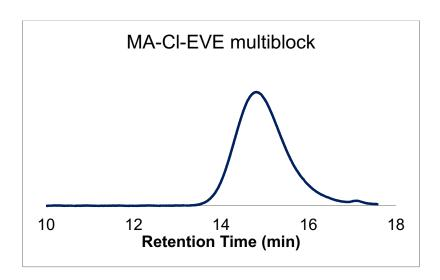
Figure 3.23. GPC trace of methyl acrylate-2-chloroethyl vinyl ether multiblock copolymer.
