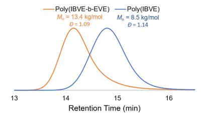
Figure 4.15. GPC traces of poly(isobutyl vinyl ether) and poly(isobutyl vinyl ether-block-ethyl vinyl ether)
