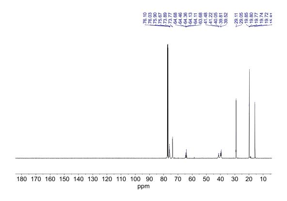
Figure 6.22. <sup>13</sup>C NMR of poly(EVE-*b*-IBVE) in CDCl<sub>3</sub> (Figure 6.3).
