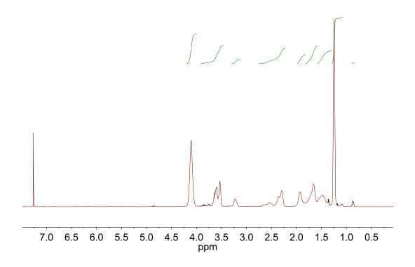
Figure 3.16. <sup>1</sup>H NMR of poly(2-chloroethyl vinyl ether-r-ethyl acrylate) ( $M_n$  = 9.0 kg/mol, D = 1.37,  $M_{n,theo}$  = 11.2 kg/mol).
