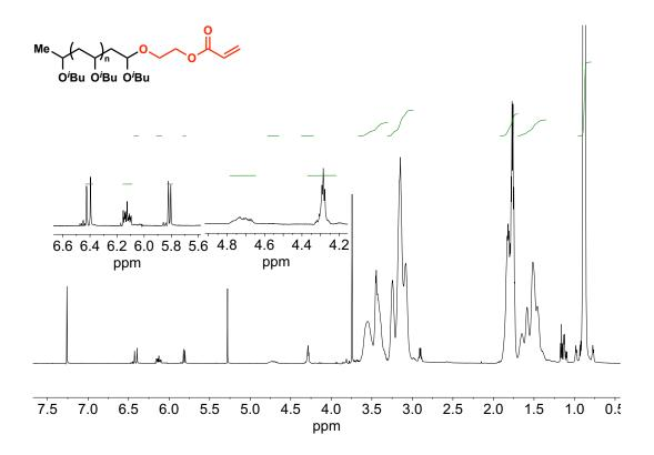
Figure 6.26. <sup>1</sup>H NMR of poly(IBVE) functionalized with 2-hydroxy ethyl acrylate;  $M_n$  (GPC) = 6.2 kg/mol;  $M_n$  (NMR) = 6.1 kg/mol.
