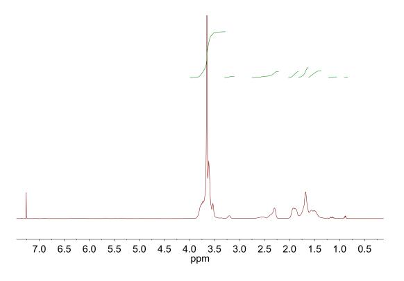
Figure 3.14. <sup>1</sup>H NMR of poly(2-chloroethyl vinyl ether-*r*-methyl acrylate)( $M_n = 6.5$  kg/mol, D = 1.41,  $M_{n,theo} = 10.3$  kg/mol).
