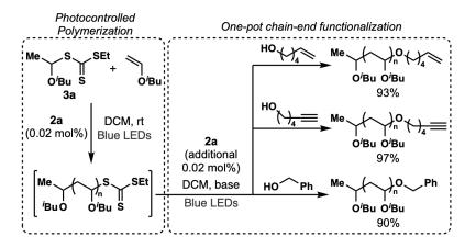
Scheme 5.1. Photocontrolled polymerization of isobutyl vinyl ether followed by chainend functionalization with alcohols in a one-pot setup (base = 2,6-di-*tert*-butylpyridine).
