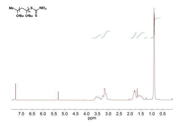
Figure 2.7a.  $^{1}$ H NMR of poly(isobutyl vinyl ether);  $M_{n}$  = 35.0 kg/mol, D = 1.30 (Table 2.1, entry 5).
