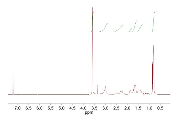
Figure 3.8. <sup>1</sup>H NMR of poly(isobutyl vinyl ether-r-methyl acrylate) ( $M_n$  = 9.3 kg/mol, D = 1.35,  $M_{n,theo}$  = 9.3 kg/mol).
