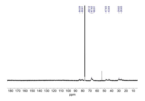
Figure 6.19. <sup>13</sup>C NMR of poly(DHF) in CDCl<sub>3</sub> (Table 6.1, entry 12).
