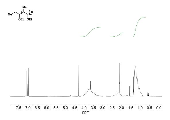
Figure 6.16. <sup>1</sup>H NMR of poly(EPE) in d8-toluene (Table 6.1, entry 10).
