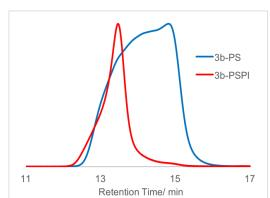
Figure 7.10. Size-exclusion chromatograms of polydisperse PS block and the corresponding PS-*b*-PI block copolymers corresponding to entries 3a,b in Figure 7.6.
