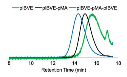
Figure 4.18. GPC traces of p(IBVE-b-MA-b-IBVE) (Figure 4.6c)
