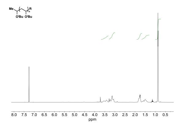
Figure 6.6. <sup>1</sup>H NMR of poly(IBVE) in CDCl<sub>3</sub> (Table 6.1, entry 1).
