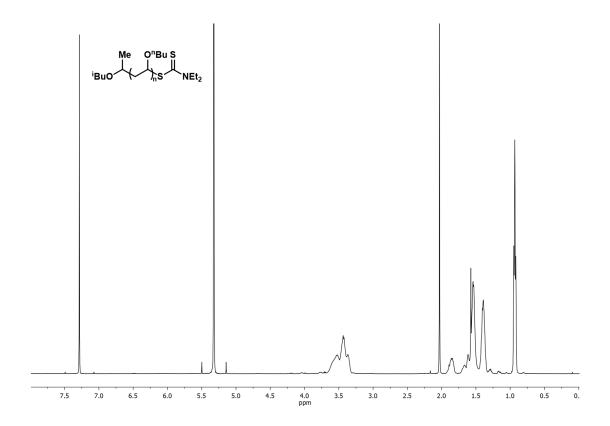
Figure 4.7. <sup>1</sup>H NMR of poly(*n*-butyl vinyl ether),  $M_n$  = 11.3 kg/mol,  $\mathcal{D}$  = 1.10 (Table 4.2, entry 1).
