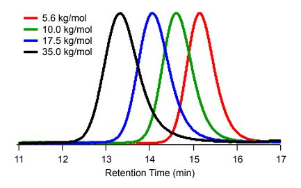
Figure 2.10. GPC traces of polymers in Table 2.1, entries 2–5.
