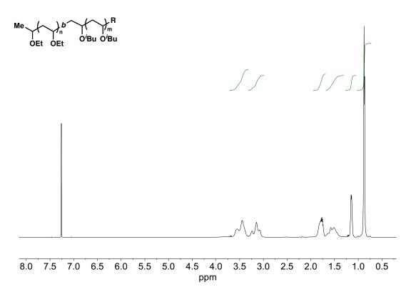
Figure 6.21. <sup>1</sup>H NMR of poly(EVE-b-IBVE) in CDCl<sub>3</sub> (Figure 6.3).
