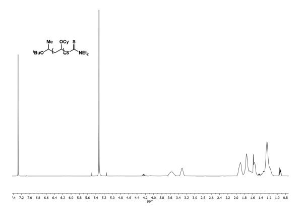
Figure 4.11. <sup>1</sup>H NMR of poly(cyclohexyl vinyl ether),  $M_n$  = 10.4 kg/mol,  $\theta$  = 1.61 (Table 4.2, entry 5).
