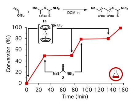
Figure 4.4. Temporal control over polymer initiation and reversible termination via the addition of FcBF<sub>4</sub> and **2**, respectively.
