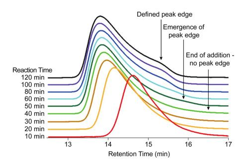
Figure 7.4. Size exclusion chromatography curves at indicated time points with a 40 min constant rate addition.
