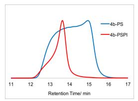
Figure 7.11. Size-exclusion chromatograms of polydisperse PS block and the corresponding PS-*b*-PI block copolymers corresponding to entries 4a,b in Figure 7.6.
