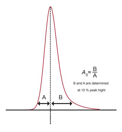
Figure 7.7. Graphical Illustration of the Calculation of Asymmetry Factor A<sub>s</sub>.
