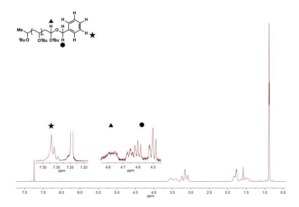
Figure 5.7. <sup>1</sup>H NMR of poly(isobutyl vinyl ether) functionalized with benzyl alcohol.
