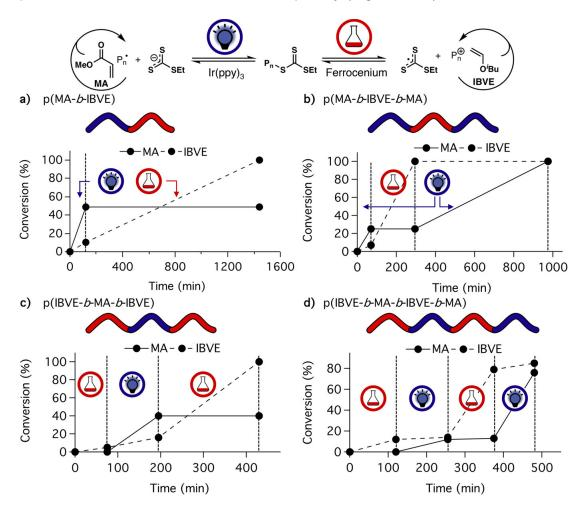
Figure 4.6. Conversion of MA (solid line) and IBVE (dashed line) over time upon applying chemically controlled cationic and photochemically controlled radical polymerization. (a) Conversion plot for poly(MA-*b*-IBVE). (b) Conversion plot for poly(IBVE-*b*-MA). (c) Conversion plot for poly(IBVE-*b*-MA-*b*-IBVE). (d) Conversion plot for poly(IBVE-*b*-MA-*b*-IBVE).
