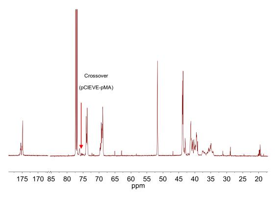
Figure 3.21. <sup>13</sup>C NMR of poly(2-chloroethyl vinyl ether-co-methyl acrylate) ( $M_n$  = 6.6 kg/mol,  $\mathcal{D}$  = 1.48,  $M_{n,theo}$  = 9.8 kg/mol).
