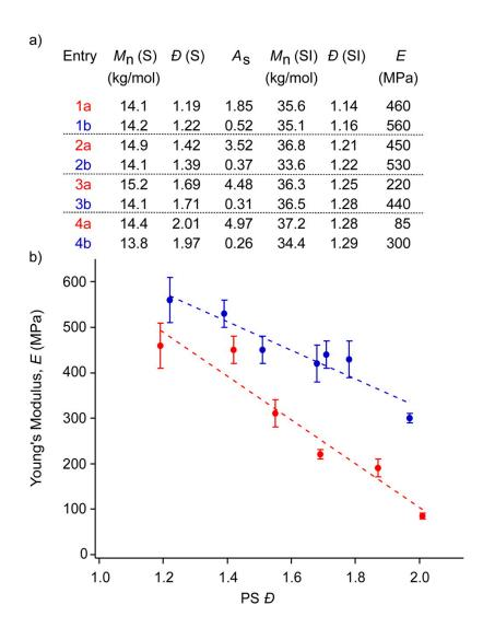
Figure 7.6. (a) Poly(styrene-block-isoprene) block copolymers with varying polystyrene (PS) MWD shapes and Young's moduli (E) determined with dynamic mechanical analysis. (b) Plot of PS  $\theta$  vs  $\theta$  (MPa): blue circles indicate PS blocks with asymmetry factor ( $\theta$ <sub>s</sub>) values of <1; red circles indicate PS blocks with  $\theta$ <sub>s</sub> values of > 1; S = PS; SI = poly(styrene-block-isoprene). Each  $\theta$  value is an average of at least four measurements.
