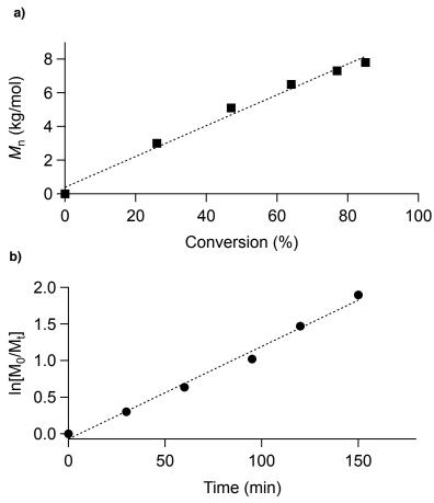
Figure 6.2. (a) The molecular weight of poly(IBVE) grows linearly with conversion. (b) A linear relationship of the change in monomer concentration with time indicates constant cation concentration throughout the polymerization of IBVE with 1.
