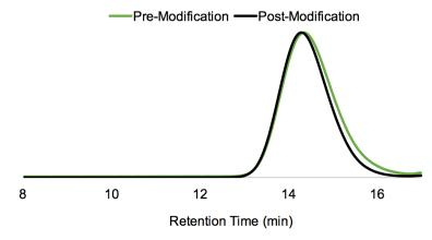
Figure 5.10. GPC traces of poly(isobutyl vinyl ether) before and after functionalization with 5-hexen-1-ol.
