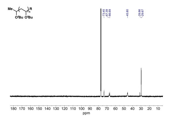
Figure 6.13. <sup>13</sup>C NMR of poly(TBVE) in CDCl<sub>3</sub> (Table 6.1, entry 8).
