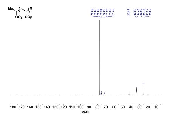
Figure 6.15. <sup>13</sup>C NMR of poly(CyVE) in CDCl<sub>3</sub> (Table 6.1, entry 9).
