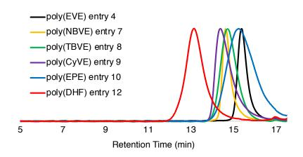
Figure 6.5. Representative GPC traces of polymers from Table 6.1.
