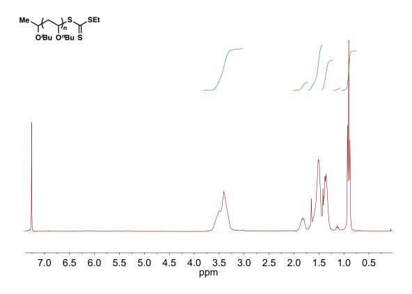
Figure 2.14a. <sup>1</sup>H NMR of poly(n-butyl vinyl ether);  $M_n$  = 5.8 kg/mol,  $\theta$  = 1.23 (Table 2.2, entry 6).
