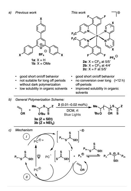
Figure 5.1. Advances in the photocontrolled cationic polymerization of vinyl ethers. a) Photocatalysts (PCs) employed in this and previous work. b) General polymerization scheme. c) Mechanism of photocontrolled cationic polymerization.
