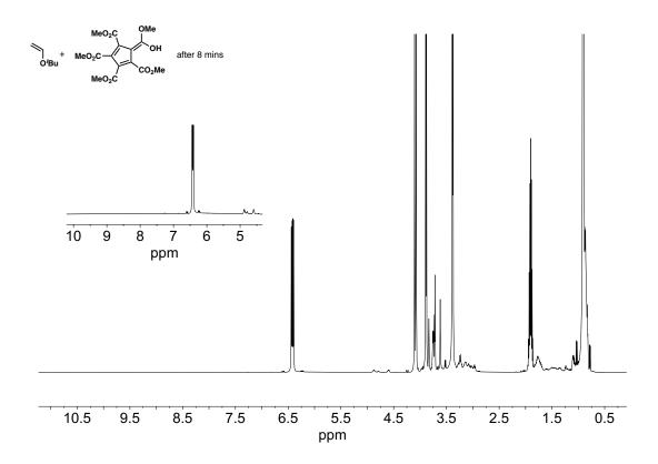
Figure 6.33. <sup>1</sup>H NMR spectrum of the IBVE and PCCP mixture after eight minutes of reaction time. Insert highlights the appearance of new resonances between 4.5 and 5.0 ppm and the absence of aldehyde and olefin resonances at the polymer chain end.
