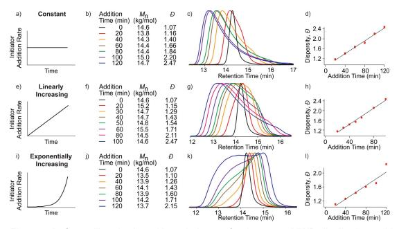
Figure 7.2. Controlling the breadth and shape of polystyrene MWD distributions with constant (a–d), linearly ramped (e–h), and exponentially ramped (i–l) rates of initiator addition (a, e, and i are representative initiator addition profiles).
