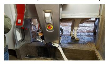
The robot will remove the cup from each quarter as it milks out. After all quarters are completed, the robot will post-dip the cow's teats
