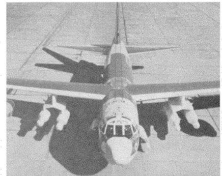
Boeing B-52H shown carrying mockups of Skybolt air-launch ballistic missiles. B-52s are also jet-fast platforms for Hound Dog guided missiles, and in addition carry regular load of gravity bombs.
