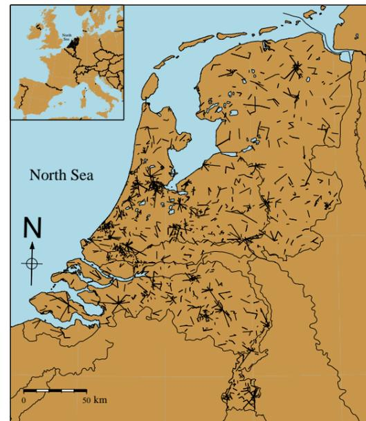
Figure 3: Part of the microwave link network of one provider.
