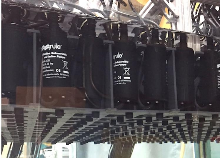
Figure 2.4: Photo of inline jet array for 16 x 16 RASJA.
