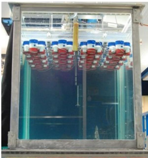
Figure 2.2: Photo of tank with 8 x 8 RASJA.
