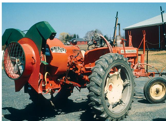
Fig. 11.7 Air blast sprayer—two-sided delivery.
