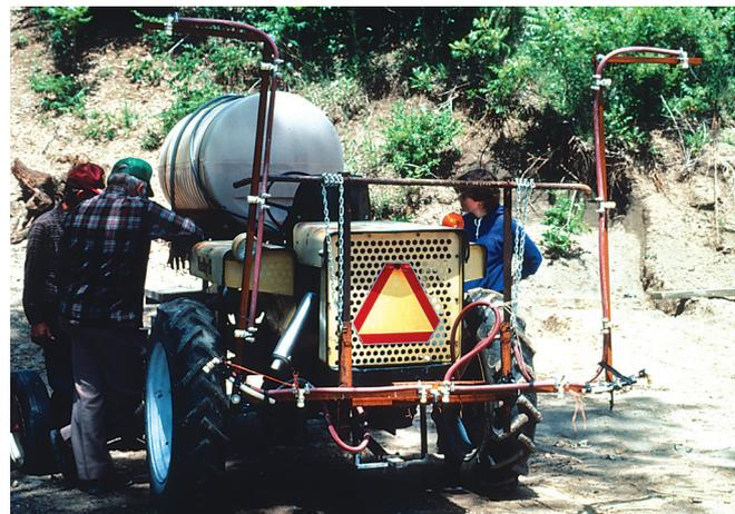
Fig. 11.10 Vertical boom sprayers.
