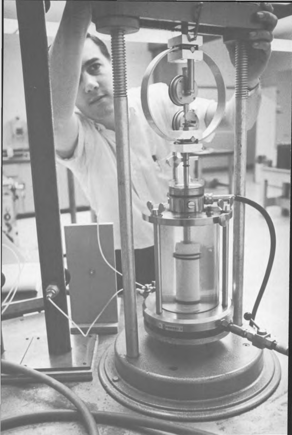
A student adjusts the triaxial soil-testing apparatus before testing a special soil sample as part of the research conducted by the Department of Geotechnical Engineering in the College of Engineering.
