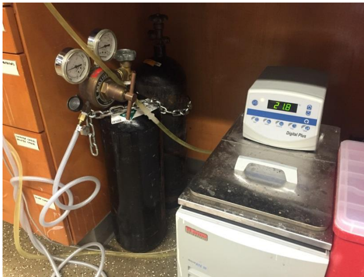
FIGURE 2.9 Air tank and water bath for the SX20. Pressurized air tanks and regulator service the SX20 drive mechanism ( left ). A temperature controlled water bath regulates the temperature of the reaction chamber by circulating fluid ( right ).
