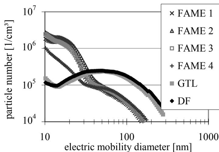
Figure 5: Particle number distributions for different fuels by SMPS; 13-mode ESC test
