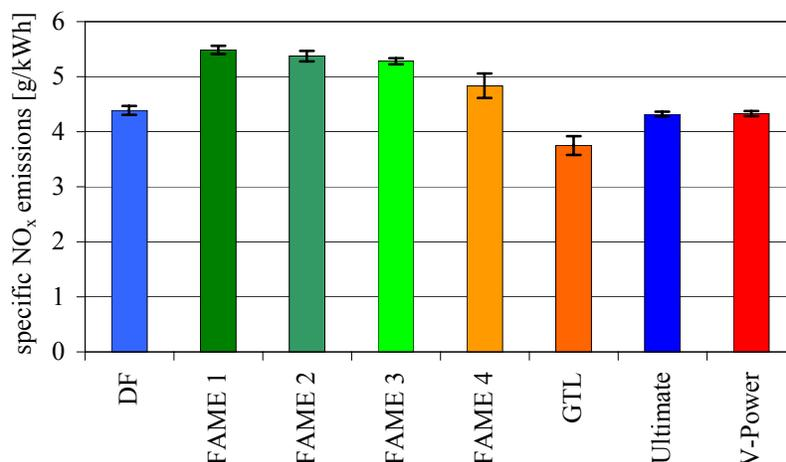
Figure 7: Specific NO<sub>x</sub> emissions for different fuels, 13-mode ESC-test
