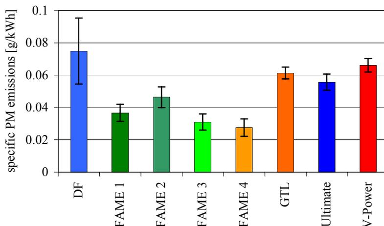
Figure 3: Specific PM emissions for different fuels; 13-mode ESC test
