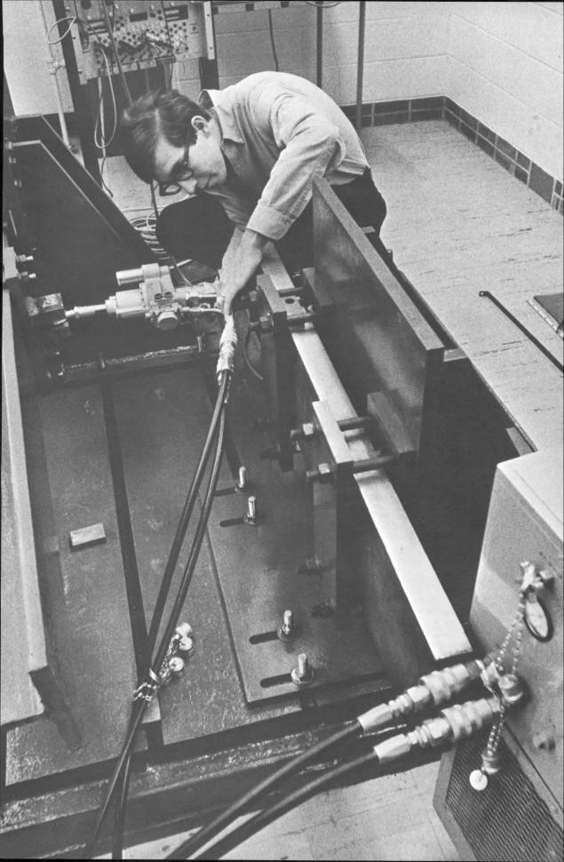
occur in reciprocating engines, have recently been formulated. Testing is made possible by a machine that was developed to simulate such conditions in the laboratory. The instability or whirl of lightly loaded bearings, dynamic cavitation, and the characteristics of the oil film between gear teeth and rolling disks are also under experimental and analytical investigation. Short bearings, eccentric loading, and temperature conditions have been extensively studied.
