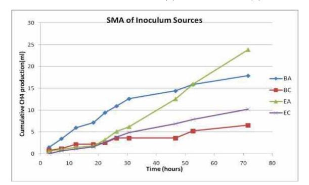
Figure 1: Methane production comparing the digester BARC (B) and Kilby's effluent (E) as inoculum sources with acetate (A) and without acetate (C).
