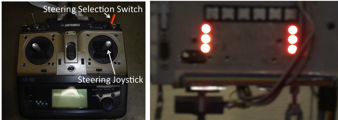
Figure 3.15: The R/C controller with steering selection switch and steering joystick labeled (left). All of Ranger's rear LED light panel flashing red to signal line tracking failure (right).
