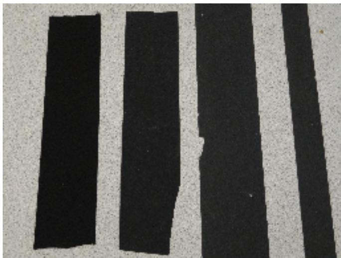
Figure 3.10: From left to right, the candidate tapes considered for use during Robots on Tour: Duvetyne tape, Shurtape, masking tape, and gaffer's tape.
