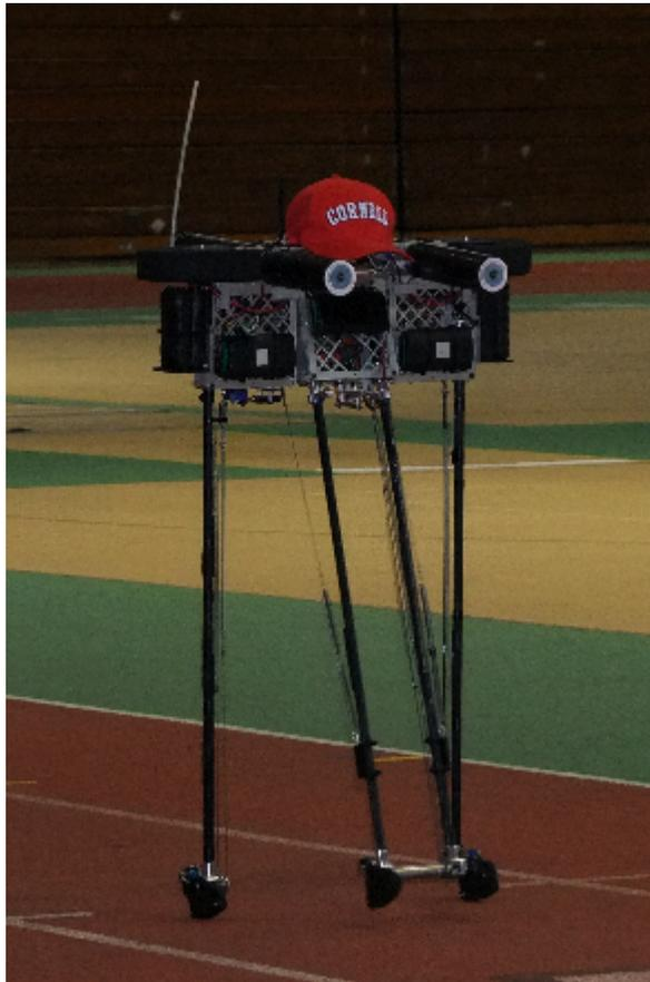
Figure 2.1: Cornell Ranger in Barton Hall during a record setting 65 km walk [1] in 2011, before this research was begun. Note the paired outer legs and paired inner legs making Ranger effectively a planar biped robot.
