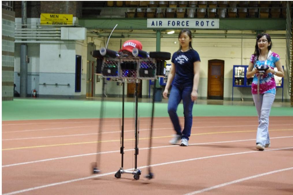
Figure 3.1: Ranger in early May of 2011 during world record setting marathon walk with undergraduate researchers Lauren Min (left) and Violeta Crow (right). Violeta is holding the R/C controller used to steer Ranger around the Barton Hall track.
