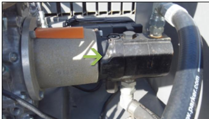
FIGURA 8. LA EMPACADORA BIGFOOT BF300 BOMBA HIDRAULICA.
