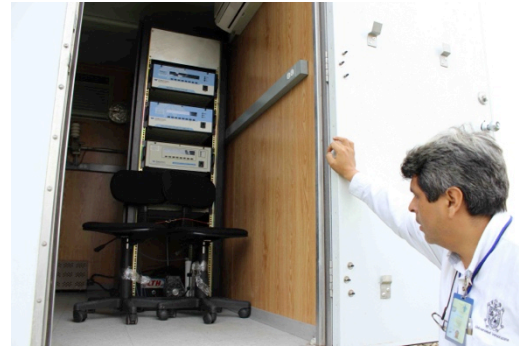
Figure 1.15. Mobile air quality-monitoring unit, Poza Rica. Photo by the author.
