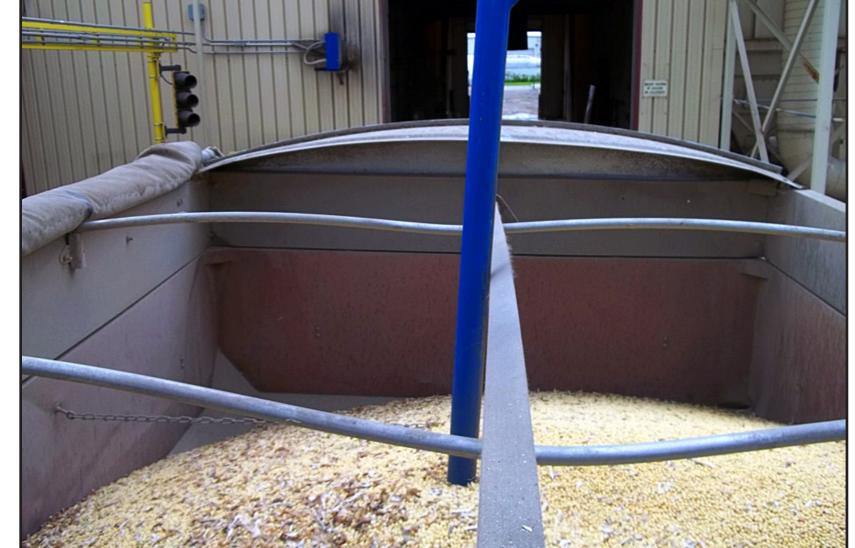
GE testing probe in a grain delivery truck
