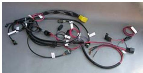
"A killer wire. Water-proof, abrasion -proof, Harley-proof wiring. Never a wiring failure since we started doing them in 1989. Automotive grade high temperature wiring with waterproof connectors, gold plated and sealed Deutsch ECU connectors, and fused peripherals, all sheathed in fiberglass wrap. Professional." (RBRacing-rsr.com).
