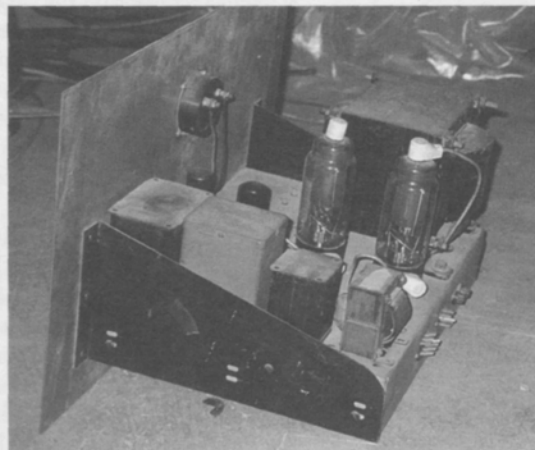
Above, Figure B. Professor Paul Ankrum's electronic regulator for the dc generator. The two glass tubes are grid-controlled mercury-vapor thyratrons in a full-wave rectifier circuit.
