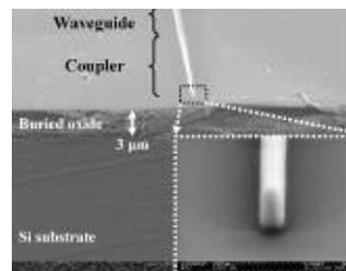
Light therefore passes from one to the other very efficiently, just as water passes efficiently from one pipe to another of equal size. Lipson's and Almeida's new design was not only significantly more efficient than most other couplers, but also much smaller and could be made using standard silicon-processing techniques.
