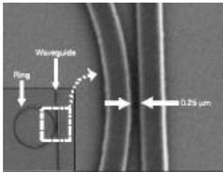
Another innovation enables light to be taken from a waveguide on a chip and projected out perpendicularly from its surface by a ring resonator (shown at left). This innovation has potential applications in computer and entertainment device displays. It is one of
