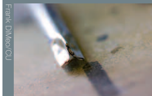
Niobium tubes used for synthesis of FC catalysts using Zintl approach
