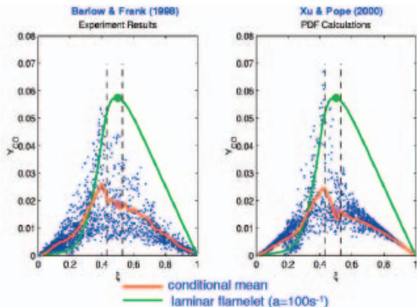
The flame being studied is a challenging test case, because the flame is close to extinction, i.e., it is almost "going out." If, on the contrary, the flame were far from extinction, then all of the points would lie close to the green line, which corresponds to a
