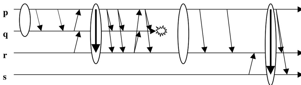
Figure 2: Multicast execution periods in Ensemble. Initially, the group consists of p and q; multicasts sent by p are delivered to q (and vice versa). r then joins and state is transferred to it. After a period of additional multicasting, q fails; s later joins and receives an additional state transfer. The period between two consecutive membership lists is denoted an "execution period".
