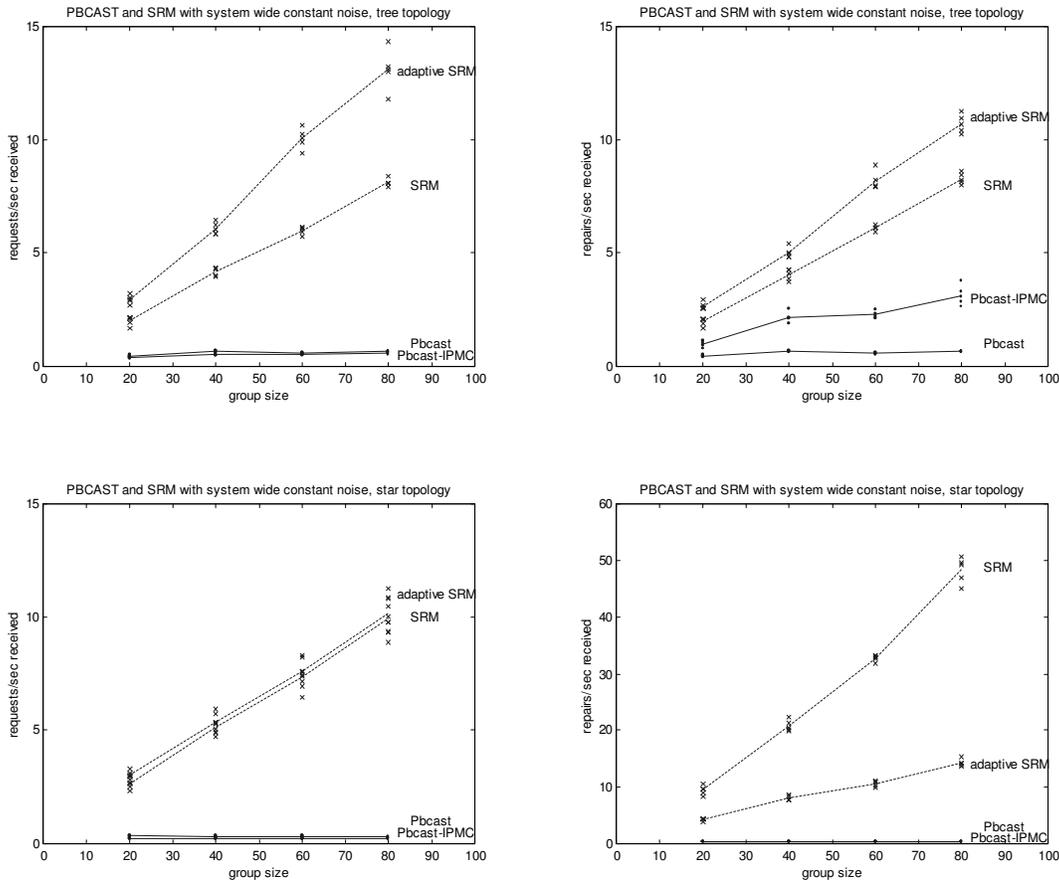
**Figure 13: Comparison of the rate of overhead messages received, per second, by typical members of a process group when using SRM and pbcast to send 100 msgs/sec with 0.1% message-loss rate on each link. Here, we look at two topologies: the same balanced 4-level tree as in Figure 12, and a star topology. In some situations, SRM can be provoked into sending multiple retransmissions (repair messages) for each request; pbcast generates lower overheads.**
