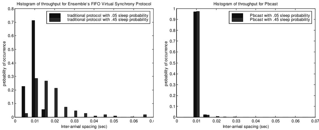
**Figure 7: Histograms of the inter-arrival spacing of multicasts in an 8-process group when using a traditional virtual synchrony protocol (left) and pbcast (right), at 75 8k-byte messages/second. The tighter distribution of pbcast supports our throughput stability claims.**
