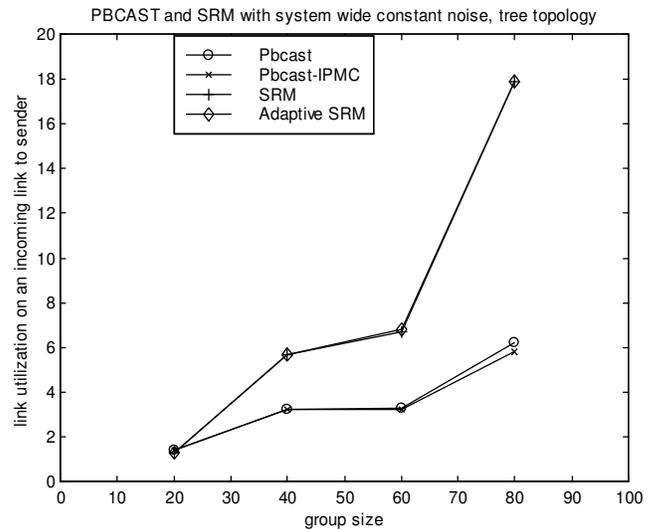
**Figure 12: SRM and pbcast. Here we compare link-utilization levels; small numbers are better. With constant noise, both protocols exhibit some growth in overheads but the scalability of pbcast is better. Here, each link had an independent packet-loss probability of 0.1%.**
