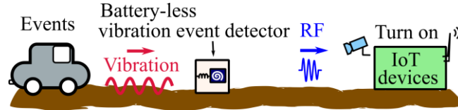
Figure 3.1: Operational scheme of the battery-less vibration event detector and RF transmitter is shown. The sensor node harvests energy from vibration and transmits RF pulses to wake up other battery powered IoT devices.
