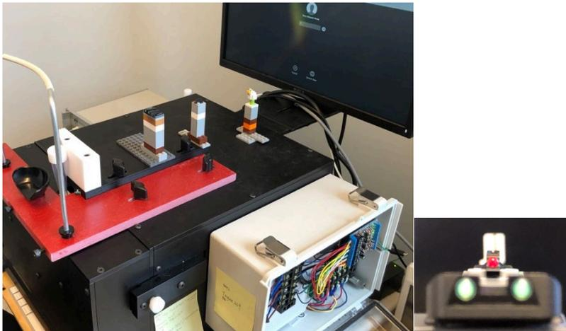
Figure 2. The auxiliary hardware in Sniff olfactometer for fixing subjects' positions: chinrest and aiming system
