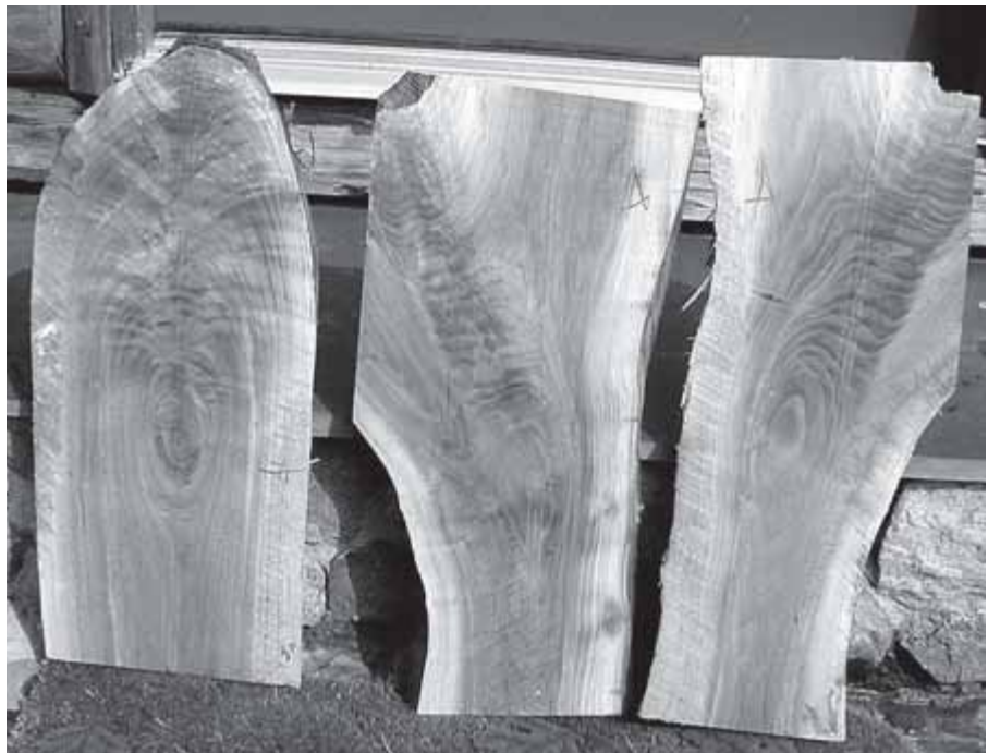
Specialty cuts such as the burl on the left and book-matched black cherry pieces on the right may be cut from a log not useful for traditional dimension lumber.
