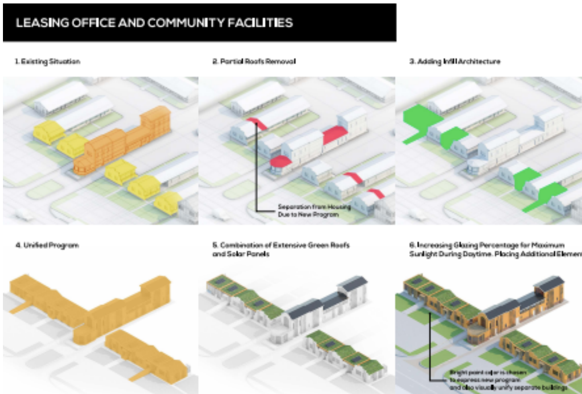
Illustration 10.9. Leasing and Community Facilities at Garden. Submission by Sadyr Khabukhayev for domestiCITY Design Competition, The City of Atlanta.
