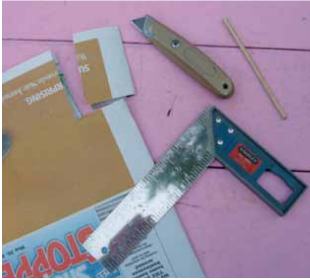
Figure E.6 Materials and tools needed to make paper tube liners.
