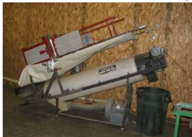
Figure 7.19 Automated cell harvesters use a series of plunger rods to punch out bee cells from Styrofoam nest blocks into a collection unit below. This particular model incorporates cell tumbling and separates excess leaf litter from the cocoons which are ejected into the garbage can at the right.
