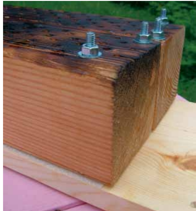
Figure E.5 Nuts, washers, bolts, drilled block, backing material, and backing board in nest block.
