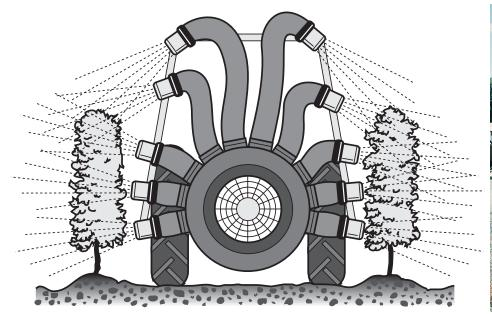
Fig. 11.8 Directed-deposition sprayer.
