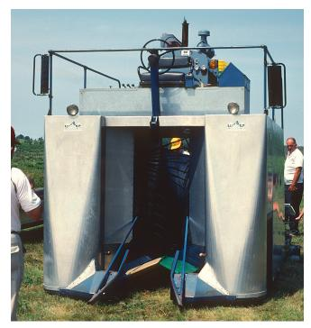
Fig. 12.1 Mechanical harvester for raspberries.
