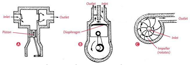
Fig. 11.2 🚯 Piston pump, 🚯 Diaphragm pump, and 🚱 Centrifugal pump.
