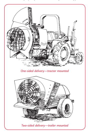
Fig. 11.6 Tractor-mounted and trailer-mounted air blast sprayers.
