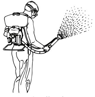
Fig. 11.14 Powered knapsack sprayer.
