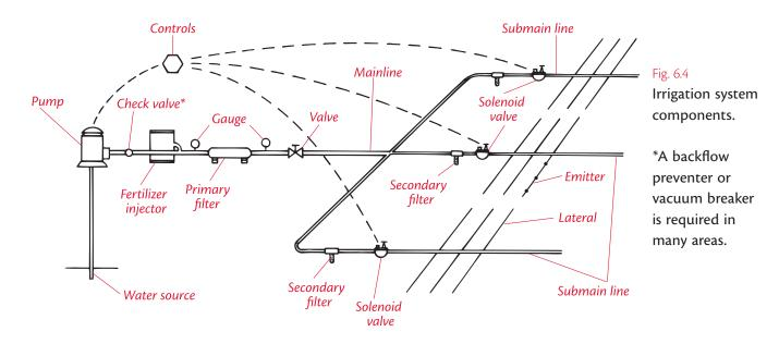
require higher pressure to operate effectively and distribute the water uniformly. Consequently, pumps for sprinkler systems generally need to be larger than those for trickle systems.
