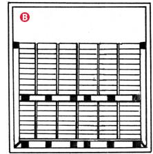
Fig. 12.3 (1) Improper loading of flats within a truck—flats are in contact with the floor and walls; (1) Proper loading—flats are not in contact with floor and walls and cold air is free to circulate.
