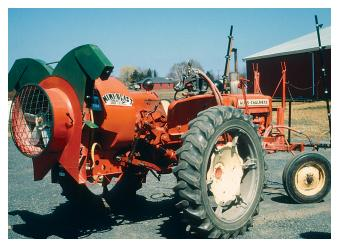
Fig. 11.7 Air blast sprayer two-sided delivery.
