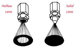
Fig. 11.3 Hydraulic sprayer nozzles.
