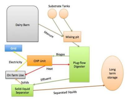
Figure 2. Lamb Farms digester flow diagram
