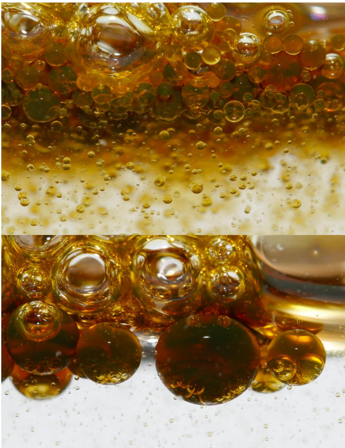
Figure 1 Photographs showing coalescence of crude oil droplets at the surface of NaCl solution shortly (top) after shaking the sample vigorously by hand and approximately 1 minute later (bottom).
