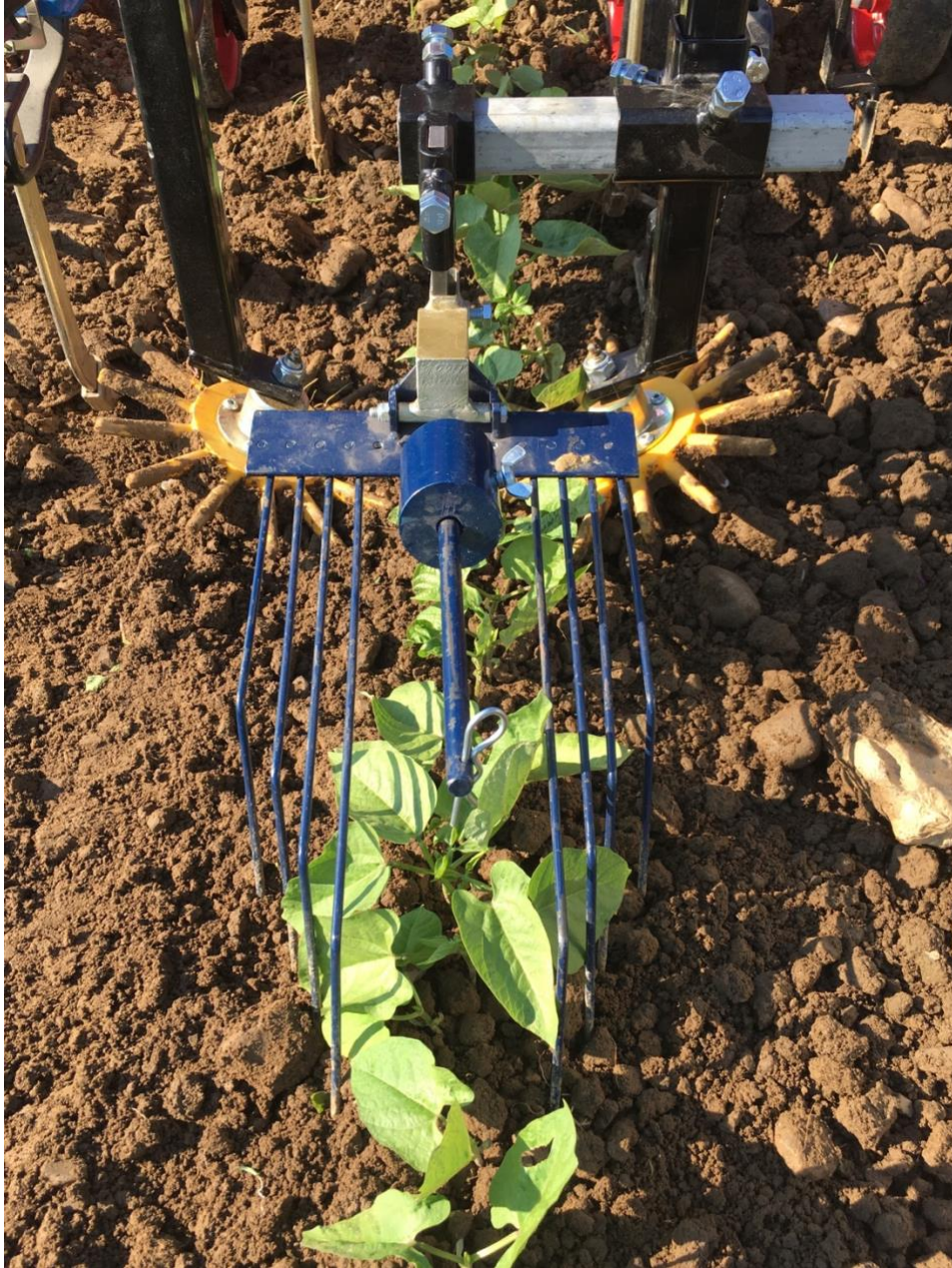
Figure 2. A row harrow (foreground) and finger weeders (background).
