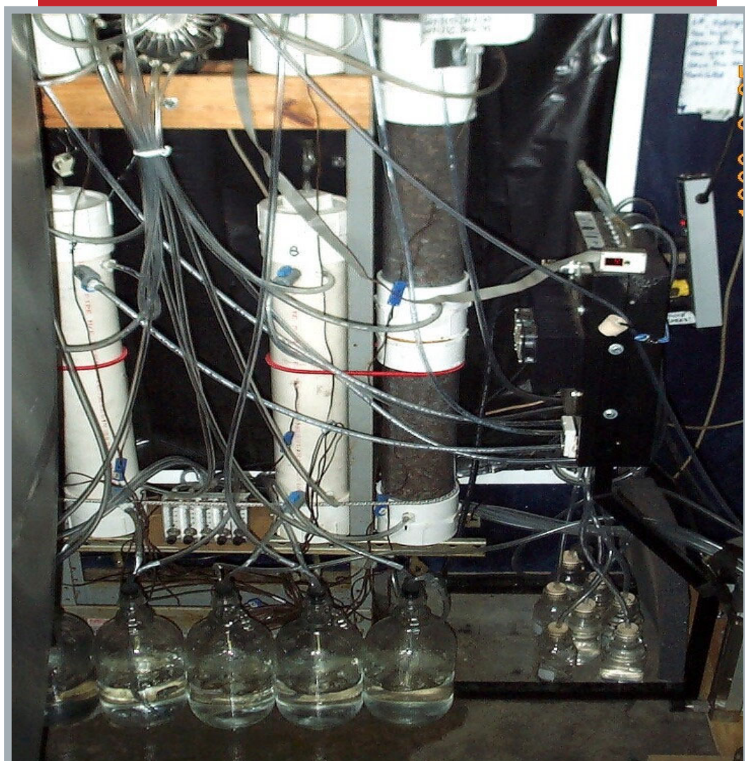
Experimental setup of bench-scale reactors for removal of hydrogen sulfide at Dairy Development International.
