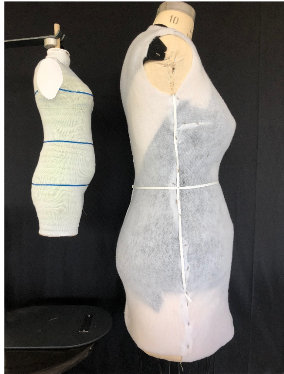
Figure 29: Custom half scale and padded full-scale dress form used by Draper 2
