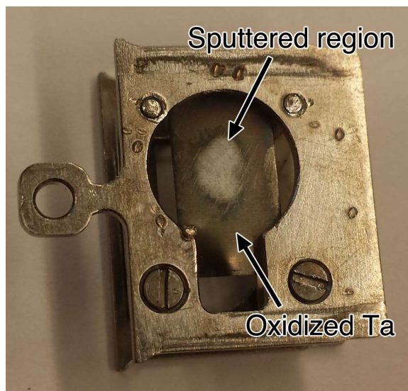
Figure 2.6: Example of a sputtered tantalum oxide film attached to a tip carrier used to align the sputter gun with the location of a tip.
