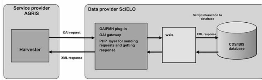
FIGURE 2 – OAI-PMH Plug-In at SciELO
