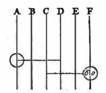
which means that an adjustment is to be made by fixing A on its axis, making a right angle with D, and that F must also make with C an angle of sixty degrees. In speaking of these angles, it should always be observed that they refer to the angles made by the parts on one of the planes of projection.
