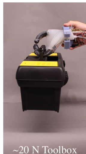
Figure 2.20 The prosthetic hand composed of silicone casted palm and injection molded hybrid fabric strain-limiting actuators can lift an approximately 20 N toolbox.
