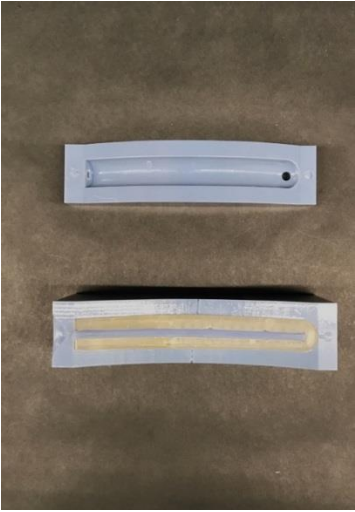
Figure 3.4 The open-channel actuator with core inserted and placed in the bottom cavity part for second-injection molding.
